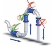
• DO NOT USE the sensor as a support to the pipe.
