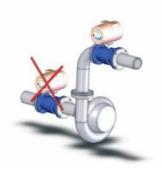
• DO NOT install the sensor in vertical pipes with free outlet or at the highest point in the pipe system
