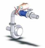
• Always install the sensor downstream the pump and NEVER upstream to avoid vacuum.
